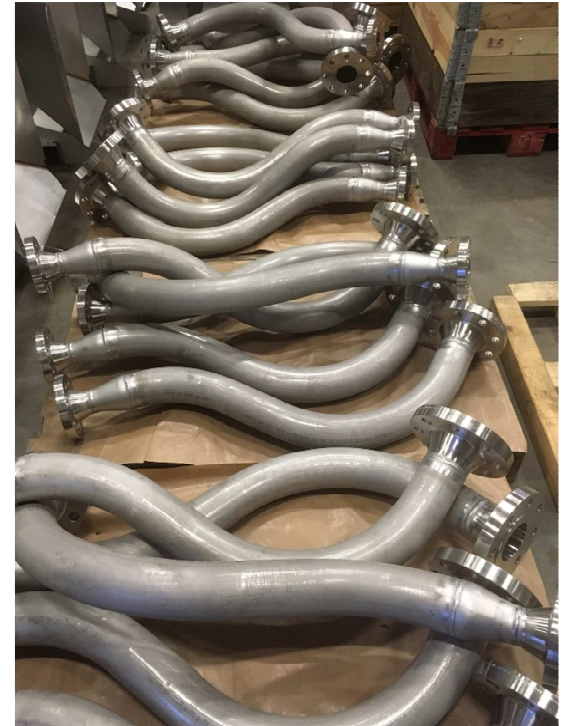
Super Duplex piping Lower Fars Project – Kuwait Oil Company
