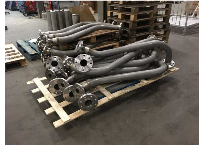
Super Duplex piping Lower Fars Project – Kuwait Oil Company
